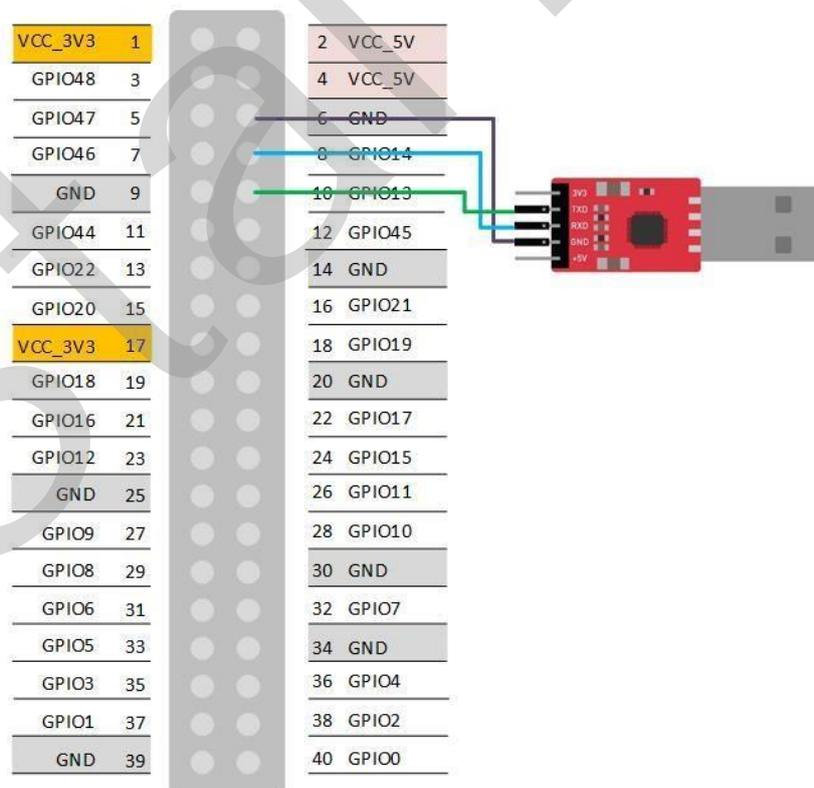
Figure 5-1 Connecting the Jumper Wires
