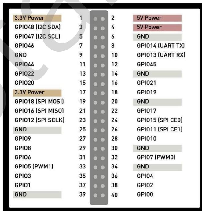
**Figure 2-3 Pinout Diagram**
