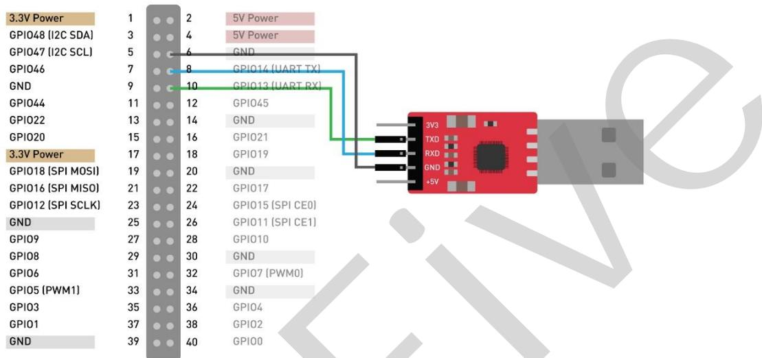
**Figure 3-10** Connecting Jumper Wires
