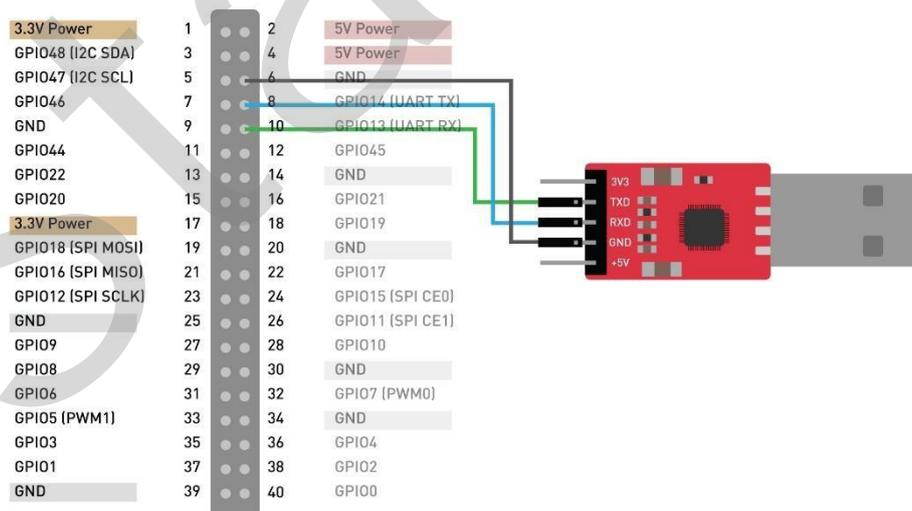
Figure 3-6 Connecting Jumper Wire
