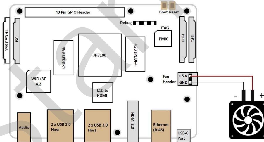
Figure 3-1 Connecting a Fan
